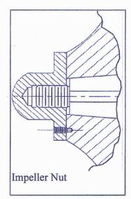
separate sleeve, eliminating the possibility of leakage under the sleeve. The impeller is locked on the shaft using a large diameter flanged acorn nut with dog-point set screw that mechanically locks in a drilled hole in the impeller. The radial bearing has been changed to a double row ball bearing and the customer is able to re-use his existing mechanical seals.
